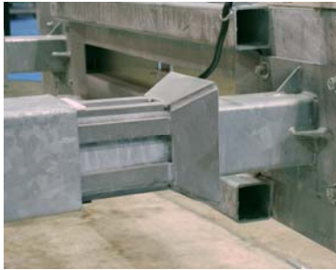
Tapered and over-sized mandrel inserted into the energy absorbing tube.
