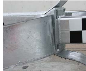
Close-up of mandrel and energy absorbing tube.
